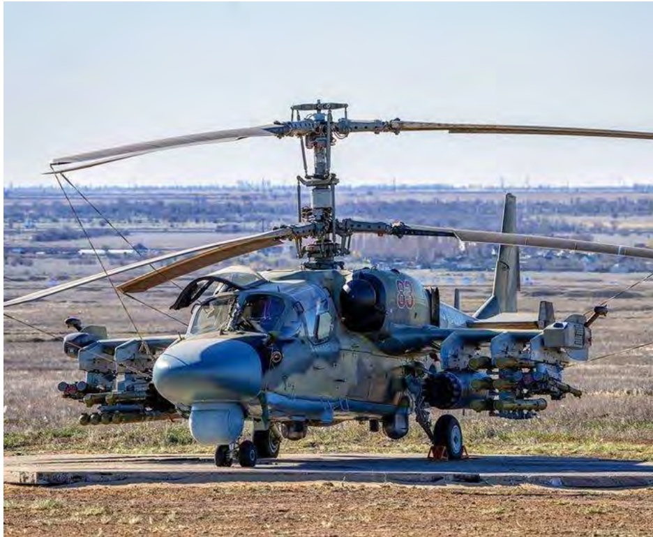
Heavily armed Ka-52 helicopter with Igla-V MANPADS, Vikhr-1 and Ataka ATGM, and B-8V-20 rocket pods for 80mm S-8 rockets. Photo: Дмитрий Мецераков
