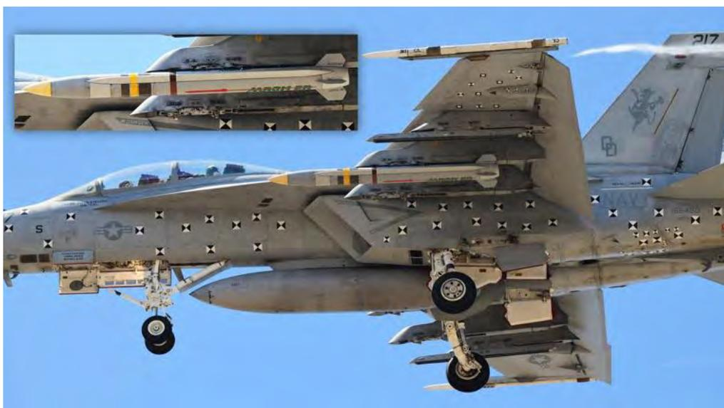
*A US Navy F/A-18F Super Hornet carrying a live AGM-88G AARGM-ER missile, with an inset showing a close-up of the missile from a different angle. © Rick Kane*
