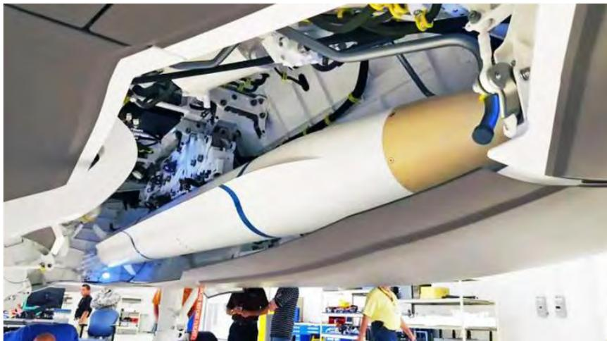
*The Drive An AARGM-ER prototype during a fit check inside the internal bay of an F-35 Joint Strike Fighter. Orbital ATK.*
