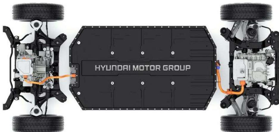
*E-GMP features an integrated drive axle, where the wheel bearings are combined with the driveshaft to transmit power.*
